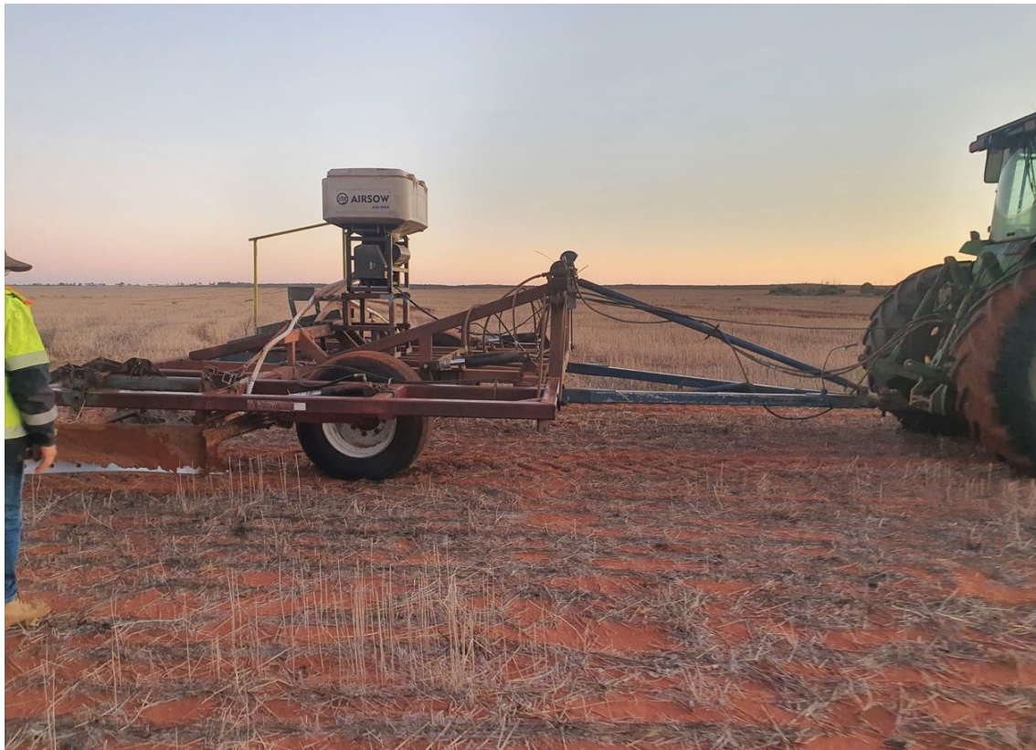
Figure 6 Rip, scalp and fertiliser machine
