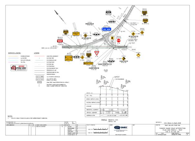
The second section (image overpage), has a Restricted Access Vehicle (RAV) Network 7.3 applied. When applying the swept paths and negotiating the 3 curves with varying Radii of 410, 550 and 435 through the section around the Buffalo Minesite, there were 4 swept path analysis (SPAs) applied. It was noted, that the Swept width of the RAV 7 configuration at 60 kph (the highest speed that the Invarion Model will permit) and is around 2.9 – 3.1m width, inside a 4m traffic lane width.
