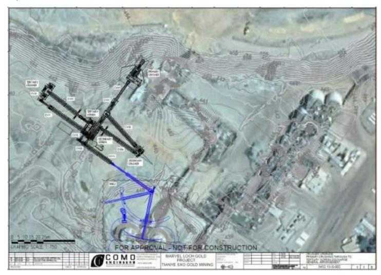
Figure 18. Layout map of crushing circuit infrastructure constructed in accordance with Condition 4, Table 6 is shown above
