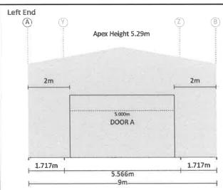
Measurements are from the outside of side girts to the inside of component opening size.
