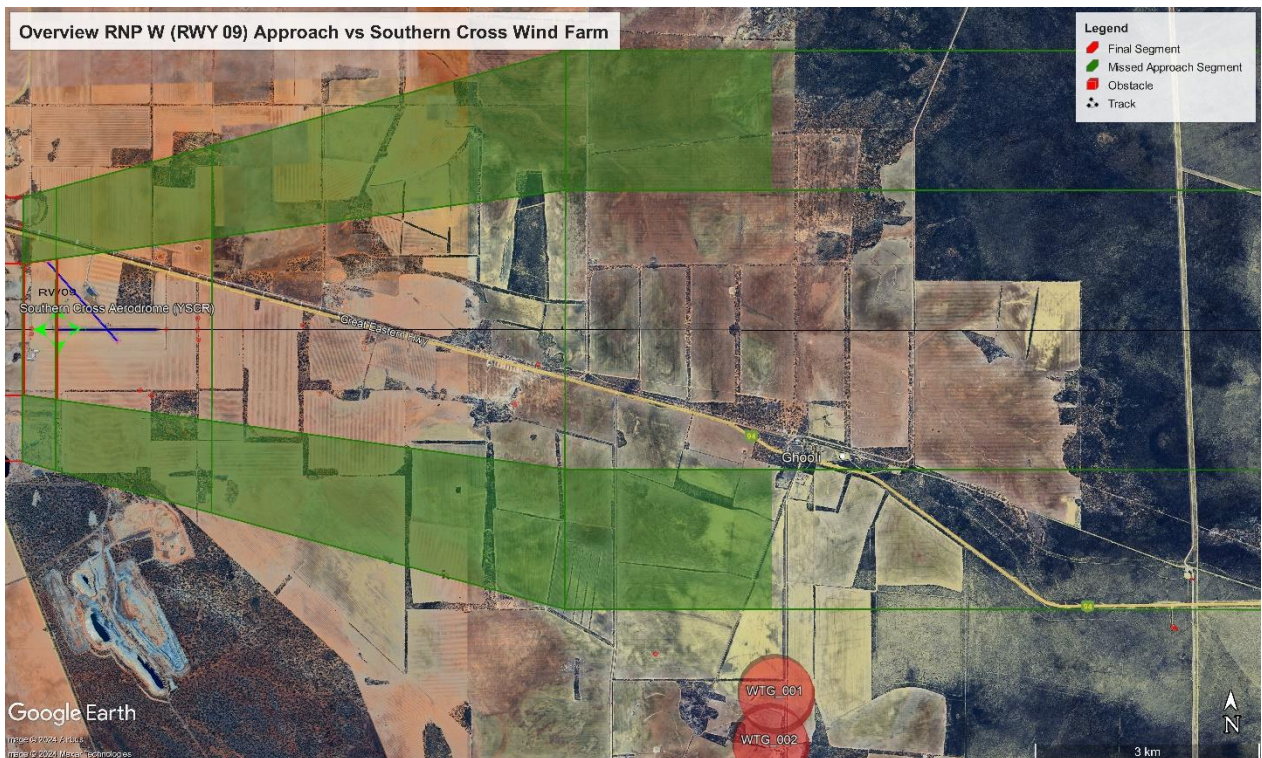
Figure 3-4 Overview RNP W (RWY 09) Missed Approach vs Southern Cross Wind Farm
