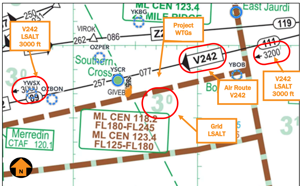
Figure 12 Grid and Enroute LSALT details
