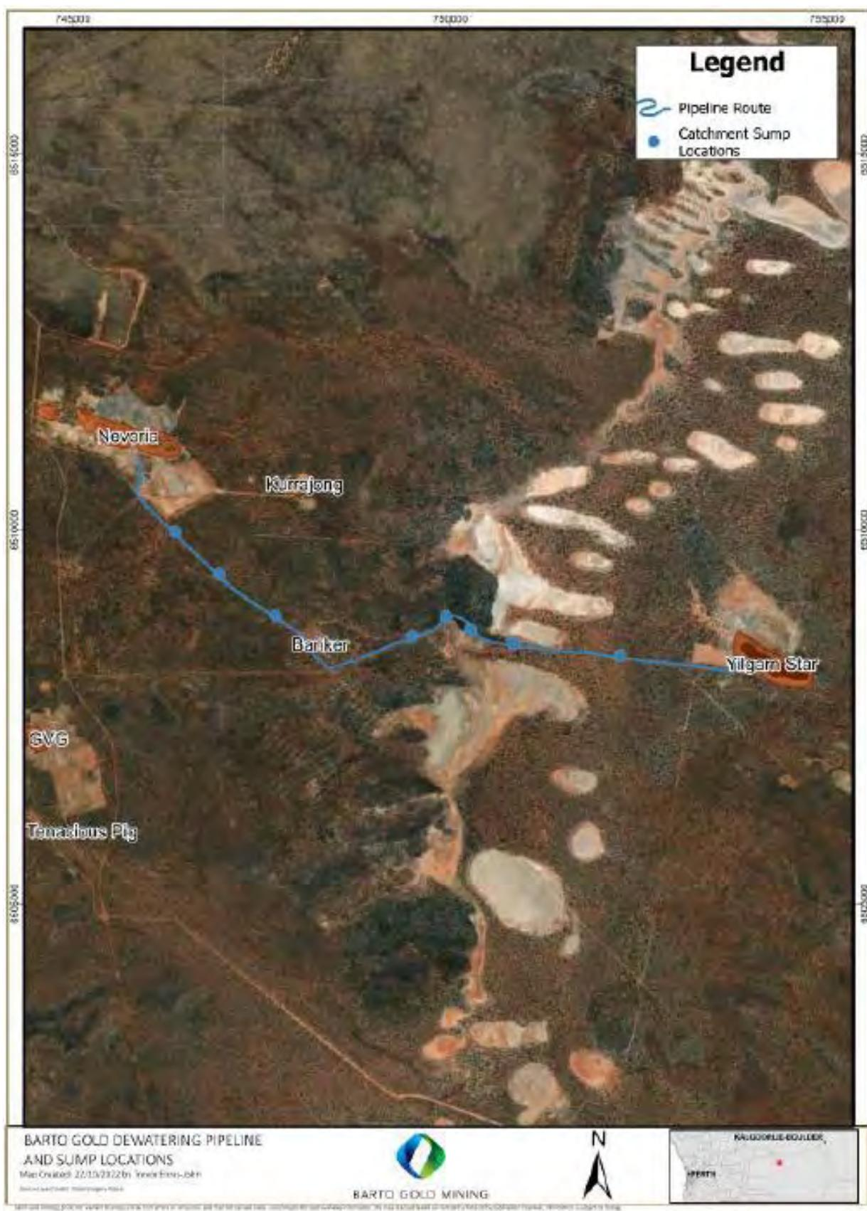
Figure 14: Location of Secondary Yilgarn Star – Nevoria pipeline with sump locations
